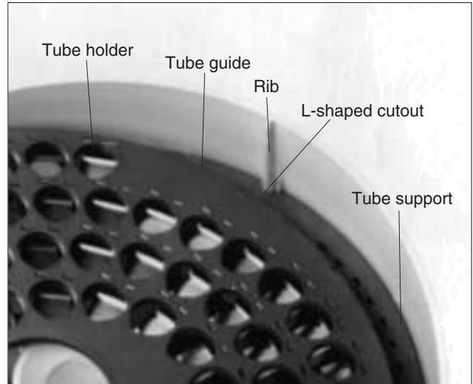
**Fig. 10.** Tube rack assembly for tube lengths
