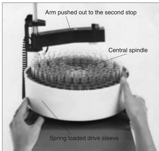
**Fig. 15.** Mounting the tube rack on to the fraction collector
