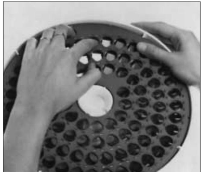
**Fig. 11.** Snapping the tube holder into place
