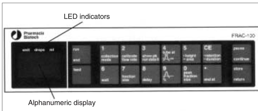
Fig. 1. Front panel.
